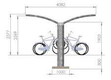
(Measurements in mm)
