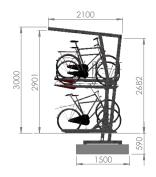
(Measurements in mm)
